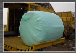
Bale height adjustable from 1.20 m to 1.60 m, thus adaption of bales to the transport vehicle, optimal use of load volume and reduction of transport costs. Fix bale diameter of 1.50 m.
