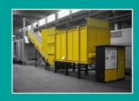
带突缘的卸料传送带,倾斜角36°,倾卸高度4.036m,位于可移动地板下方的功能箱,涵盖液压站、冷却器、液压元件以及电控箱 / Discharge conveyor with grouser belt, discharge height approx. 4.036 m at 36°. Functional cabinet with hydraulic aggregate, cooler, hydraulic components and control cabinet below pushing floor.
